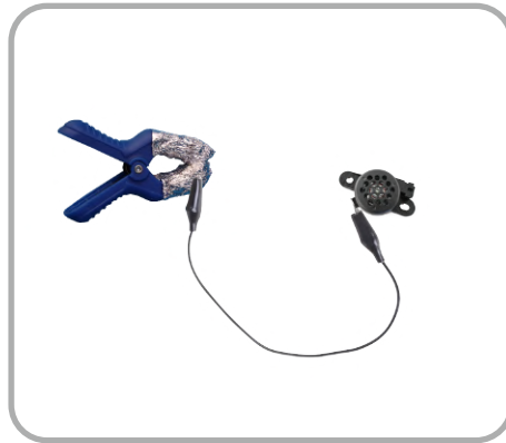
Connect one aluminum foil to a wire of the buzzer.
