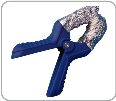
Wrap the ends of the pliers in aluminum foil, separated from each other
